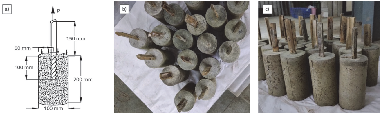
Figure 5. a) Schematic representation of pull-out sample; b) Actual pull-out test specimen
